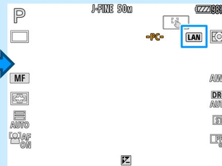
Open the live view. If the **LAN** icon is white, the network has been recognized by the camera. ◦
